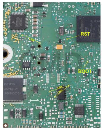
The pads marked above to make contact with the probe.
