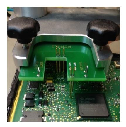
**3.** Disconnecting: To safely disconnect the probe from the ECU, you must first remove the power supply on the adaptor cable (see adaptor cable overview on page 1). Once the power cable is disconnected it is safe to lift the BDM frame and probe away from the ECU.
