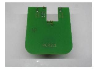
**1. Description:** This adaptor set can be used for unlocking and programming Simos Continental PCR2.1 ECU's. It fits in most BDM positioning frames. Included in the kit is the PCR probe and an ECU cable.
