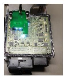
If lighting is required you can connect a 12V power supply to the jack on the probe (this only powers the LED's and not the ECU).
