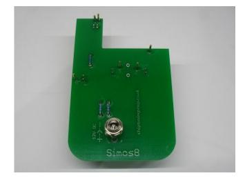
**1. Description:** This adaptor set can be used for unlocking and flashing Simos 8 ECU's. It fits in most BDM positioning frames. Included in the kit is the Simos 8 probe and an ECU adaptor cable.
