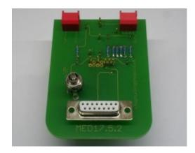
**1. Description:** This probe can be used for programming VAG MED17.5.2 Bosch ECU's. It fits in most BDM positioning frames and is fitted with LED's for accurate alignment on the ECU. The "Boot" resistors and the "Reset" lines can be disconnected via a switch to read out the password of protected ECU's. The LED's can also be switched off.
