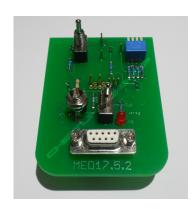
**1. Description:** This probe can be used for programming VAG MED17.5.2 Bosch ECU's. It fits in most BDM positioning frames and is fitted with LED's for accurate alignment on the ECU. The "Boot" resistors and the ignition feed can be switched. **With this adapter, there is no need to solder at all.**
