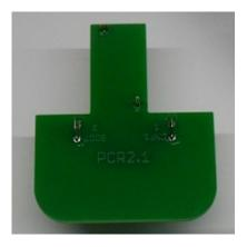
**1. Description:** This adaptor set can be used for unlocking and programming Simos Continental PCR2.1 ECU's. It fits in most BDM positioning frames. Included in the kit is the PCR probe and an ecu adaptor cable set.
