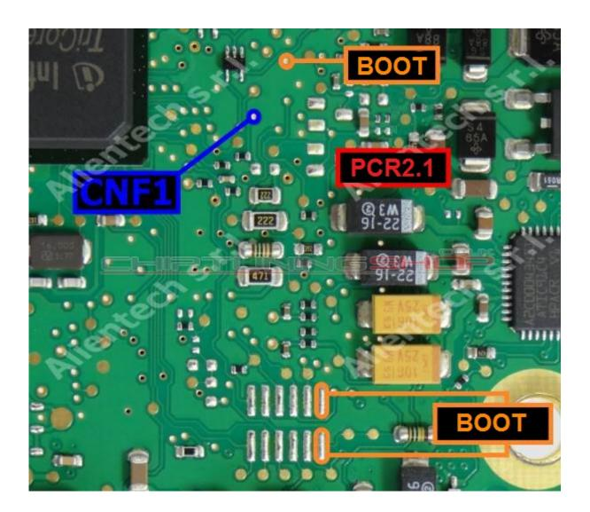
The pads marked in Blue and Orange have to make contact with the probe.
