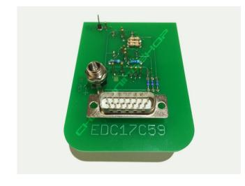
1. Description: This probe can be used for programming Opel / Vauxhall EDC17C59 ECUs with K-TAG or Trasdata. It fits in most BDM positioning frames and is fitted with LEDs for accurate alignment on the ECU. Included in the kit is the probe and 2 cables.
