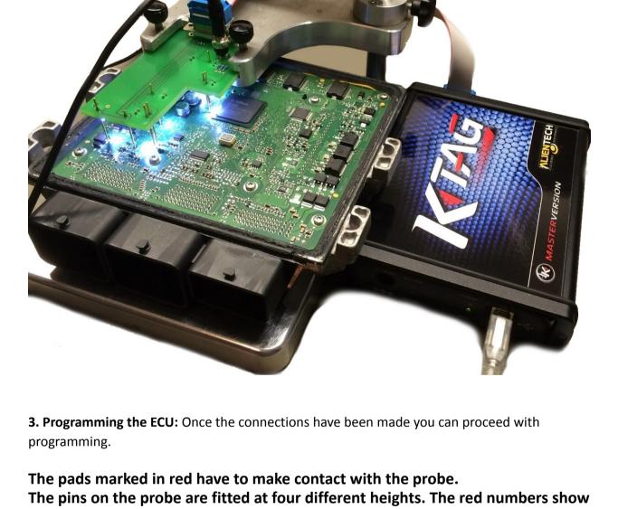
the 4 stages in which the probe hits the ECU.
