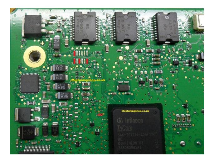
The pads marked in red have to make contact with the probe.
