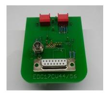
**1. Description:** This probe can be used for programming DEUTZ / FENDT / VALTRA EDC17CV44 and EDC17CV56 Bosch ECU's. It fits in most BDM positioning frames and is fitted with LED's for accurate alignment on the ECU. The "Boot" resistors and the "Reset" lines can be disconnected via a switch to read out the password of protected ECU's. The LED's can also be switched off.
