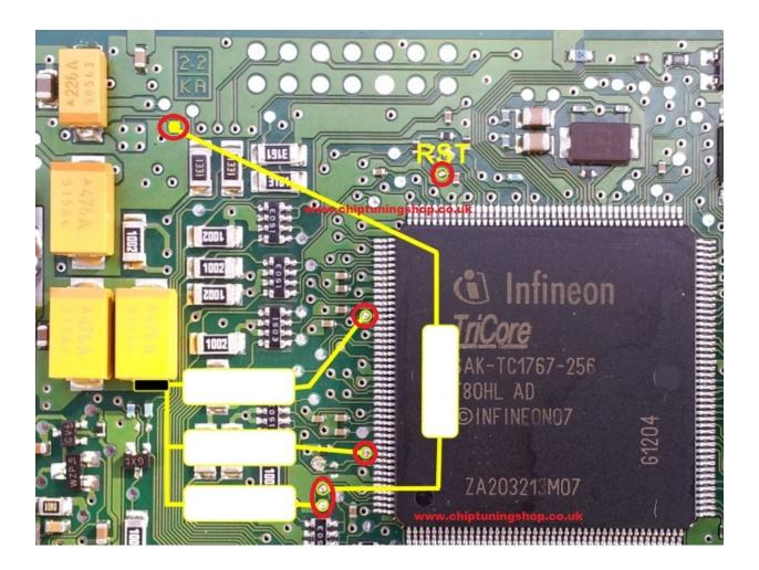
The pads circled in RED have to make contact with the probe.
