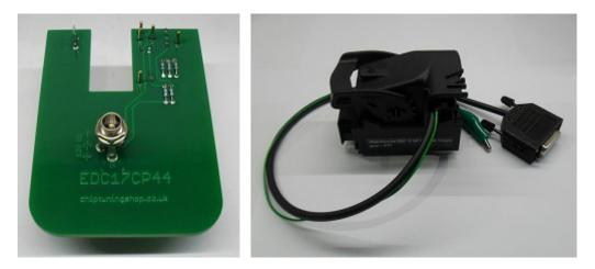
**1. Description:** This probe can be used for programming VAG EDC17CP44 Bosch ECU's. It fits in most BDM positioning frames and is fitted with LED's for accurate alignment on the ECU. Included in the kit is the probe and an ECU adaptor cable.
