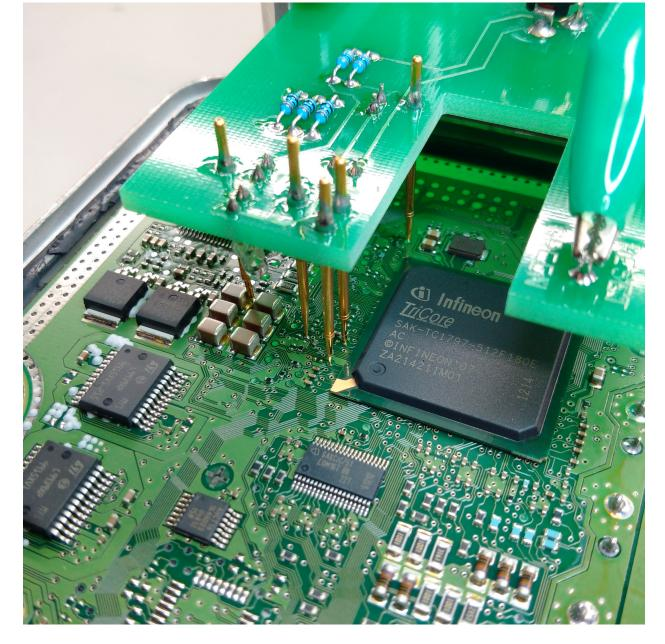
Attach the green crocodile clip on the ECU cable to the probe "RESET" connection as pictured. You can now program the ECU.
