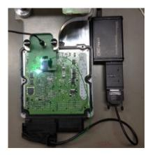
**4. Programming the ECU:** Place the probe into the BDM frame retaining bracket and tighten the screws.
