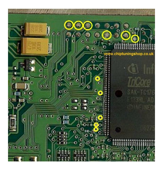
The pads marked in yellow have to make contact with the probe.
