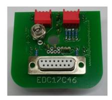
**1. Description:** This probe can be used for programming VAG EDC17C46 Bosch ECU's. It fits in most BDM positioning frames and is fitted with LED's for accurate alignment on the ECU. The "Boot" resistors and the "Reset" lines can be disconnected via a switch to read out the password of protected ECU's. The LED's can also be switched off.
