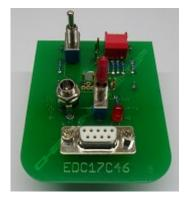
**1. Description:** This probe can be used for programming VAG EDC17C46 Bosch ECU's. It fits in most BDM positioning frames and is fitted with LED's for accurate alignment on the ECU. The "Boot" resistors and the ignition feed can be switched. **With this adapter, there is no need to solder at all.**
