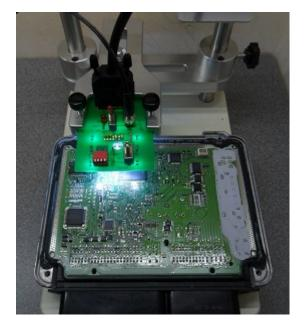
**3. Reading password: (This step is only necessary for TP8+).** Lift up the Boot DIP switches **(D)** as shown in the adapter overview on page 1 and set the Ignition switch **(E)** to the **"ON**" position, you can now read the password.
