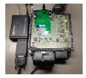
If lighting is required you can connect a 12V power supply to the jack on the probe (this only powers the LED's and not the ECU). It is possible to use the CMD power supply to power the LED's temporarily whilst aligning, once aligned you can return the power supply back into the CMD interface.
