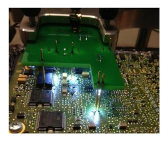
**3.** Disconnecting: To safely disconnect the probe from the ECU, you must first remove the power supply! Once disconnected it is safe to lift the frame and probe away from the ECU.
