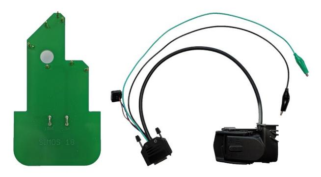
**Description:** This adaptor set can be used for programming Simos 18 ECU's. It fits in most BDM positioning frames. Included in the kit is the probe and an ECU cable.
