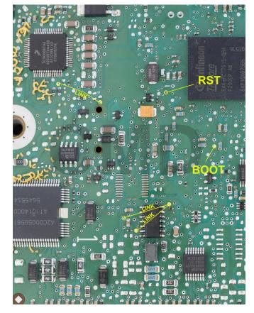
The pads marked above to make contact with the probe.
