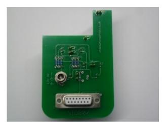
**1. Description:** This probe can be used for programming Continental SID807 TC1797 ECUs. It fits in most BDM positioning frames and is fitted with LEDs for accurate alignment on the ECU. Included with the probe is a 5mm perspex sheet.
