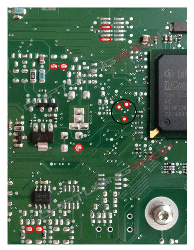
The pads marked in red have to make contact with the probe. The probe hits the 3 circled pins first. If they are in their designated position, then you can move the adaptor towards the ECU and connect to the remaining pads.
