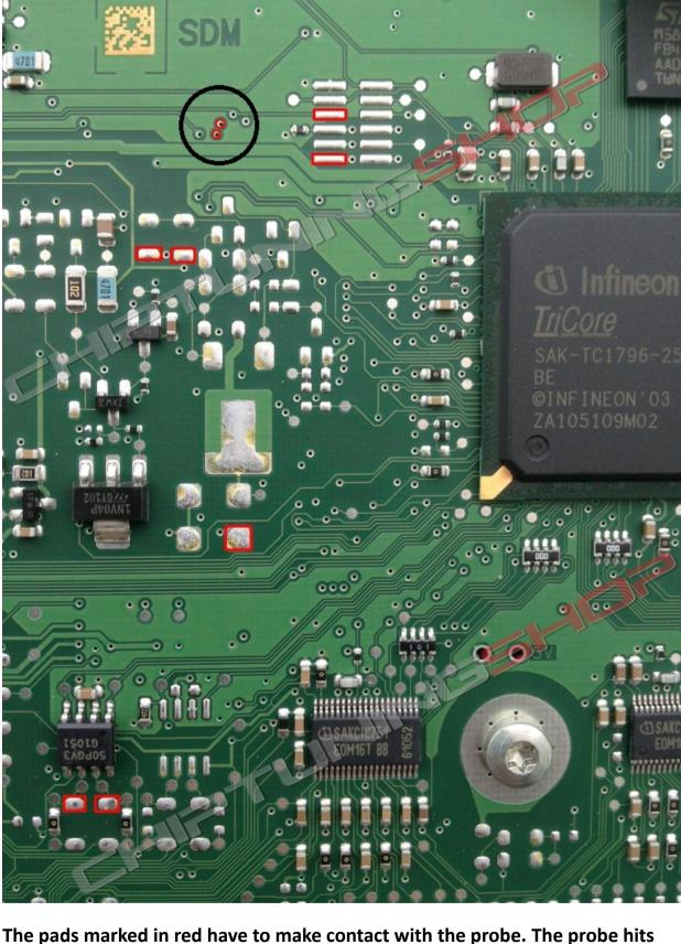
the 2 circled pins first. If they are in their designated position, then you can move the adaptor towards the ECU and connect to the remaining pads.
