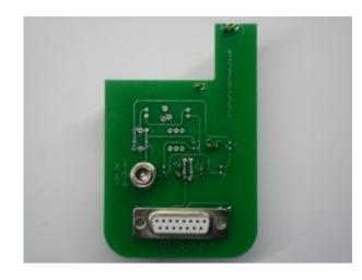
**1. Description:** This probe can be used for programming Continental SID807 TC1796 ECUs. It fits in most BDM positioning frames and is fitted with LEDs for accurate alignment on the ECU. Included with the probe is a 5mm perspex sheet.
