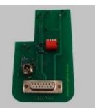
**1. Description:** This probe can be used for programming Continental SID208 ECUs. It fits in most BDM positioning frames and is fitted with LEDs for accurate alignment on the ECU. The "Boot" resistors and the "Reset" lines can be disconnected via a switch to read out the password of protected ECUs. Included with the probe is a 5mm perspex sheet.
