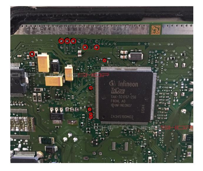
The pads marked in red have to make contact with the probe. The pins on the probe are fitted at different heights to allow easier connection in 3 stages.
