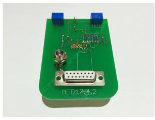
**1. Description:** This probe can be used for programming PSA MED17.4.2 Bosch ECU's. It fits in most BDM positioning frames and is fitted with LED's for accurate alignment on the ECU. The "Boot" resistors and the "Reset" lines can be disconnected via a switch to read out the password of protected ECU's.
