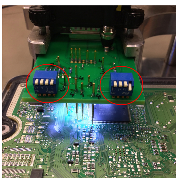
Probe set to password reading mode.
